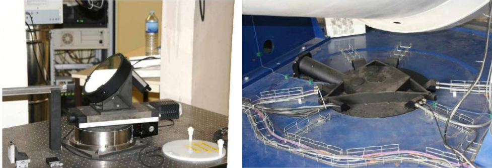
Figure 4. 200 mm high energy Fold mirrors; distribution bench on the left.
